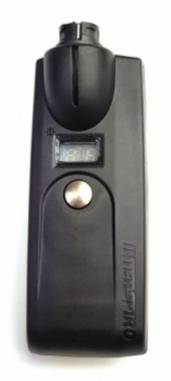
Spirocom RAI (Radio Adapter Interface) is a radio adapter that is easily attached directly to the long range radio. The Spirocom system is built to handle the difficult conditions at a fire scene and still deliver high quality sound.
