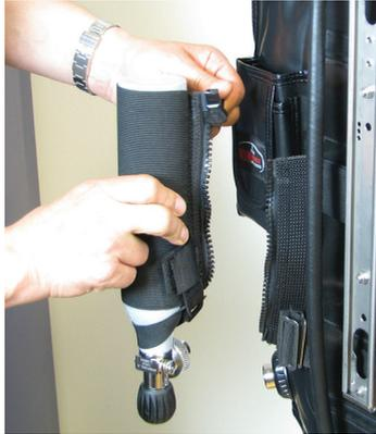
3. Open the cylinder valve shortly to drain the inside connector piece from possible water contained in there.
