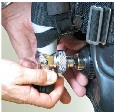
2. Remove the rescue air inflation cylinder by unzipping it from the BC.
