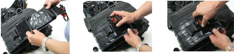
If you are using a large amount of weight, it is recommended to re-insert the weight pockets after the donning procedure, immediately before the dive, to reduce the overall weight of the system being handled.
