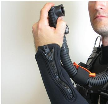
As you descend and when you reach your desired depth you will need to add air to your Divator Rescue BC by pressing on the filling button of the power inflator to attain “neutral” buoyancy.
