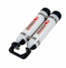
The low profile of the Divator steel pack configuration allows the diver to work with less water resistance in fast-flowing currents. With the cylinder valve facing downward there are no valves or hoses behind the diver's head, greatly reducing snagging hazards. The valve down configuration allows the diver to reach the valve and all hoses even when wearing a restricting dry suit. The handle makes it is to carry the cylinder pack and also acts as protection for the regulator.
