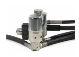
The Divator MKIII regulator has an extremely high flow capacity. The design ensures that the intermediate pressure leading to the breathing valve is stable and is not affected by pressure variations in the air supply or the depth of the dive.
