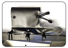
When the holder has been mounted, slide in the battery canister and guide the cable through both elastic cord loops.
