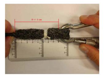
If the loop is not correct, the communication Line shall be sent to Interspiro for corrective actions.
