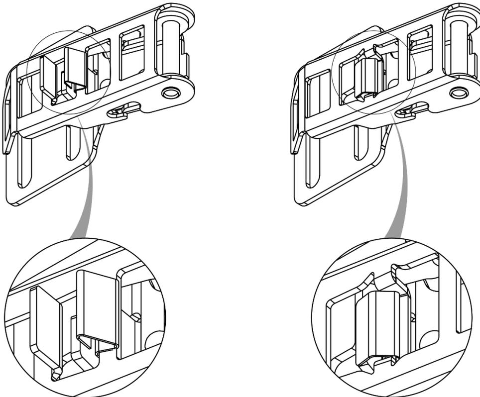
The locking tab on the cylinder strap buckle has been redesigned. See pictures.
