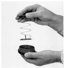
**e)** Remove the sealing disc from the diaphragm assembly.
