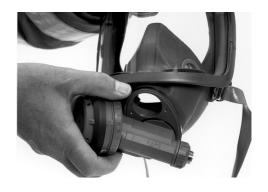
**2.** Mount the cover, speech cone or radio interface (Savox) in the face mask. Tighten the screws by hand.
