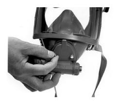
**3.** Turn the breathing valve clockwise so that it comes away from the bayonet fitting and pull the valve outwards.
