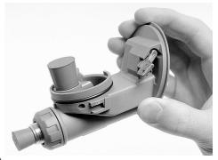
**d)** Remove the positive pressure spring and the guide disc from the cover.
