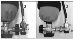
valve by simply pushing them together. When the escape cylinder is pressurised the quick coupling is locked and not possible to disconnect. With the escape SCBA evacuated of air the quick coupling can be disconnected by pushing the locking ring and then removing the regulator unit from the cylinder valve.
