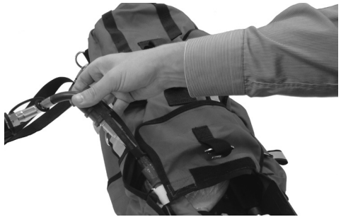
Route HP/medium pressure hoses through slot
