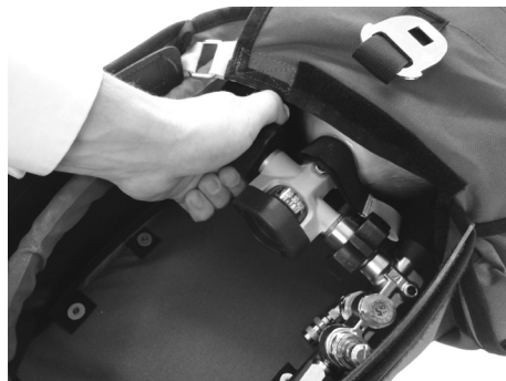
Opening cylinder valve
