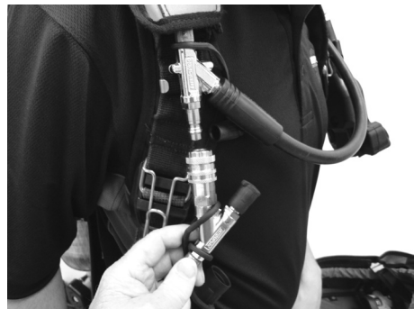
Connecting to SCBA airline connector
