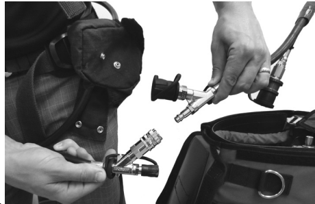
Connecting to SCBA Buddy Breathing hose (if equipped)
