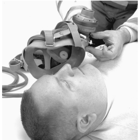
Turning on positive pressure
