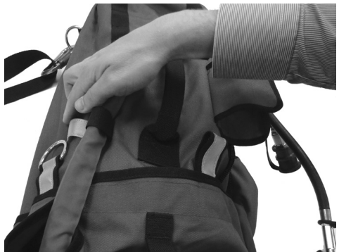
Secure hoses with the velcro strap
