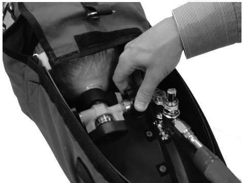
Tighten RIT regulator handwheel or connect the quick coupling
