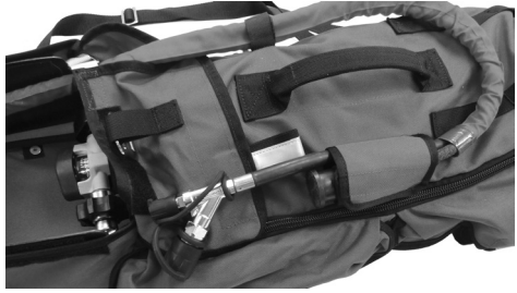
Secure the ends of hose assemblies with velcro flap
