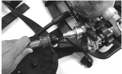
Connecting the charging whip
