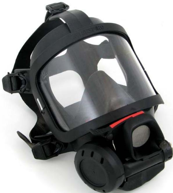
The mask is equipped with an ambient air hatch enabling the user to have the mask fully donned and still breathe ambient air to save the compressed air in the cylinder. With a very simple operation, a push on the hatch cover, the air from the cylinder is activated.
