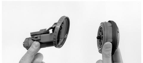
**b)** Seal off the connection nipple and the inlet channel with rubber plugs.
