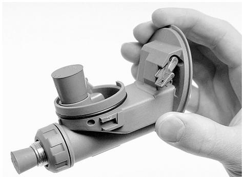
d) Remove the positive pressure spring and the guide disc from the cover.
