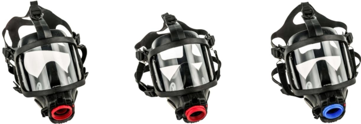
Every part of the mask is optimised to give an unrestricted and strong flow of air through the mask and directed straight up onto the visor. With this design fogging of the visor has been minimized and any fogging from stand-by mode is quickly flushed away.
