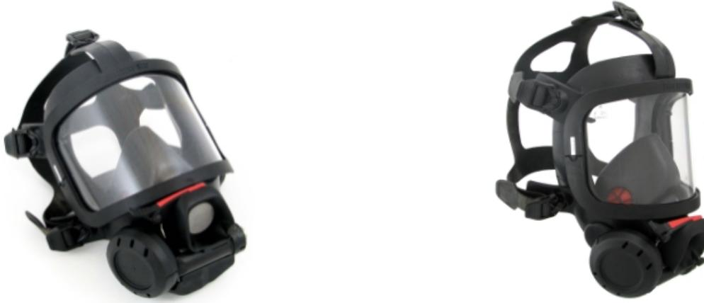
The S-H mask is equipped with an ambient air hatch enabling the user to have the mask fully donned and still breathe ambient air to save the compressed air in the cylinder. With a very simple operation, a push on the hatch cover, the air from the cylinder is activated.
