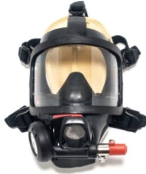
The mask is equipped with an ambient air hatch enabling the user to have the mask fully donned and still breathe ambient air to save the compressed air in the cylinder. With a very simple operation, a push on the hatch cover, the air from the cylinder is activated.
