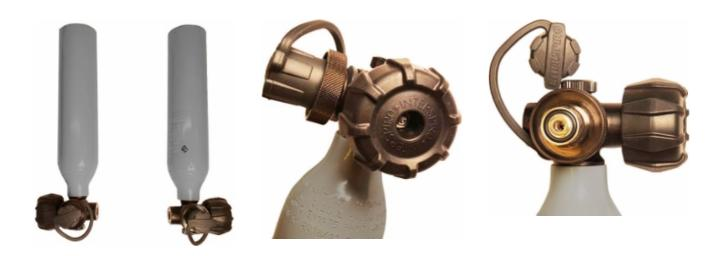
The Divator Inflation cylinder has a valve that is operated in a 90° angle to the cylinder. This design gives a more safe opening procedure compared to traditional inflation cylinders. By turning at this angle the cylinder itself is kept from rotating even by soft fabric pockets. When turning the hand wheel you are sure to open the valve instead of just rotating the cylinder.
