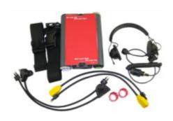
The Ibsophone wired under water communication system provides excellent voice communication between divers and the surface attendant. One surface unit can communicate with two divers and the divers can communicate with each other. The Ibsophone contributes to a high degree of diver safety and also improves the underwater work. When connectors are removed from the amplifier the unit is switched off.
