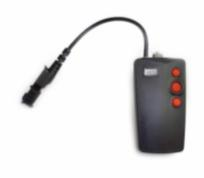
Spirocom GRA (Generic Radio Adapter) is a radio adapter that can be connected to most wellknown long range radios on the market. The Spirocom system is built to handle the difficult conditions at a fire scene and still deliver high quality sound.
